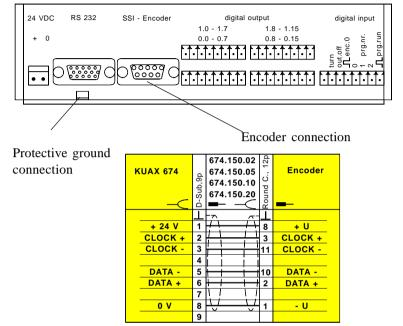
The following connecting cables and cable lengths are available:
