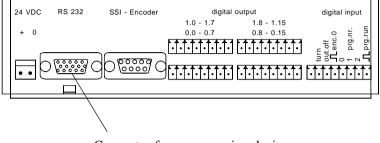
Connector for programming device
