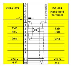
The cable is firmly attached to the PG 674. The 24 V DC voltage is supplied by the control device.
