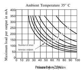
The diagram shows the maximum load of the individual outputs for differing loads on an output group for an ambient temperature of  $35^{\circ}$  C (outside the KUAX 674). If the temperature rises by 15 K, the maximum possible load drops by ~25%.
