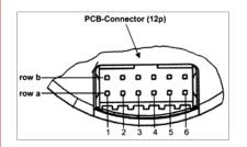
12 pin PCB connector manufacture Berg, type Minitek
