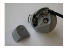
12 pin PCB connector manufacture Berg, type Minitek Screen is connected over a length of 10 mm with encoder housing.
