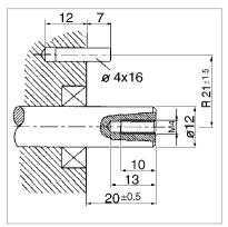
Dimensions in mm also apply for shaft-Ø 10 or 14 Mounting = E (mounting with center screw)
