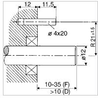
Dimensions in mm also apply for shaft-Ø 10 or 14 Mounting = D, F (Clamping ring) Preparation of the machine flange <sup>1</sup> (all mounting versions):
