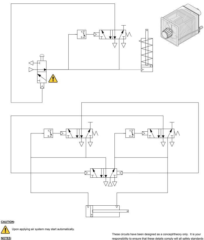
Clean dry non lubricated air to be used. Timers should never be adjusted while in operation. Pressures should not exceed timer specification.
