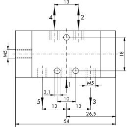
Air jet detectors are used for contact sensing of parts and tools and often used for sensing delicate components. A stream of air is sent from a nozzle, as an object touches off the nozzle the stream is blocked causing back pressure which operates the valve. When using the M5 threaded nozzle, any length of tube can be used, however, the tube length and volume will determine the valve switch time.
