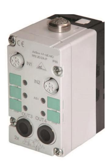
The **AirBox 1** has 2 inputs and 2 pneumatic outputs. You can wire up the input sockets directly with sensors (PNP, via M12 plugs) in 2- or 3-wire connection. The sensors are
