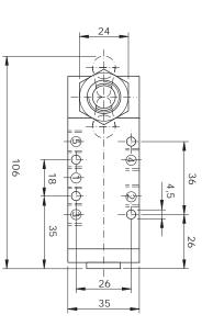
Flow rate orifice 6mm kv=9,7 l/min
