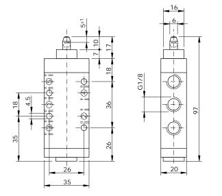
Flow rate orifice 6mm kv=9,7 l/min
