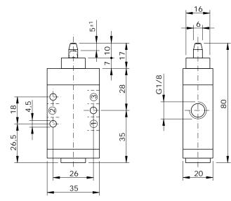
Flow rate orifice 6mm kv=9,7 l/min
