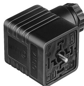
Plug-in socket Z803 Screw joint PG 9 for lead diameter 4.5 - 7 mm
