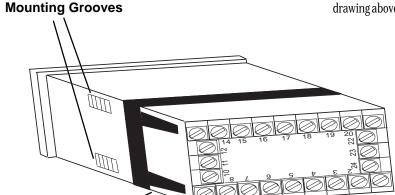
The instrument can be mounted in a panel with a thickness of up to 6mm. The cutout(s) should be made based on the recommended panel opening illustrated in the drawing above.
