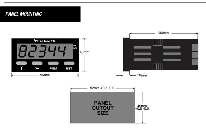
Mounting Grooves drawing above drawing drawi
